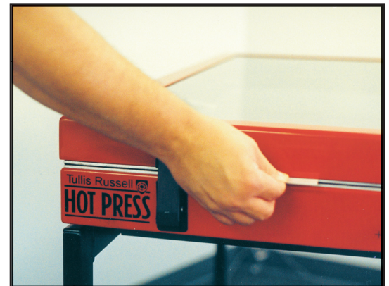
Illustration 15B: Tugging on each strip to determine vacuum seal.
