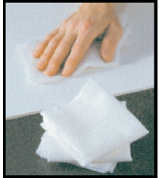
Illustration 13A: Using TacCloth to wipe down foam board.
