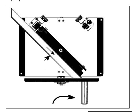
The disk should be coming *down* onto the top of the mitred edge, forcing it into the table and fence.
